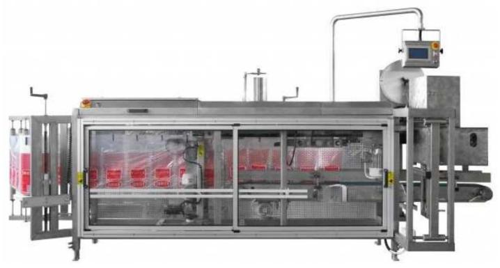
The Horizontal Sealing Machine is ideal for packing hard vegetables or loose products into PE Bags on reel. Ideal for products such as carrots, potatoes, onions etc. Two different types, for Premade PE Bags (AP Models) & Centre-Fold / Half Tube Film (APF Models)
